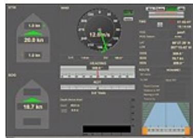
Navi-Conning is a software and hardware system, which is intended for the processing and recording of parameters supplied via different channels from external sources of information. This system will considerably simplify the work of watch officers by permanently providing valid information on the operation of ship systems. The software features base screen views and allows the possibility of custom-made individual screens. The soft instruments can be repeated across the boat network.
